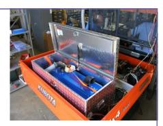
The ATV pictured is equipped with an LDS unit. The LDS is shown housed in a toolbox that is placed in the back of this vehicle. The air is sampled from the front of the vehicle and transported to the LDS through a 2-inch diameter hose. Power to the LDS is from vehicle battery or auxiliary batteries.
